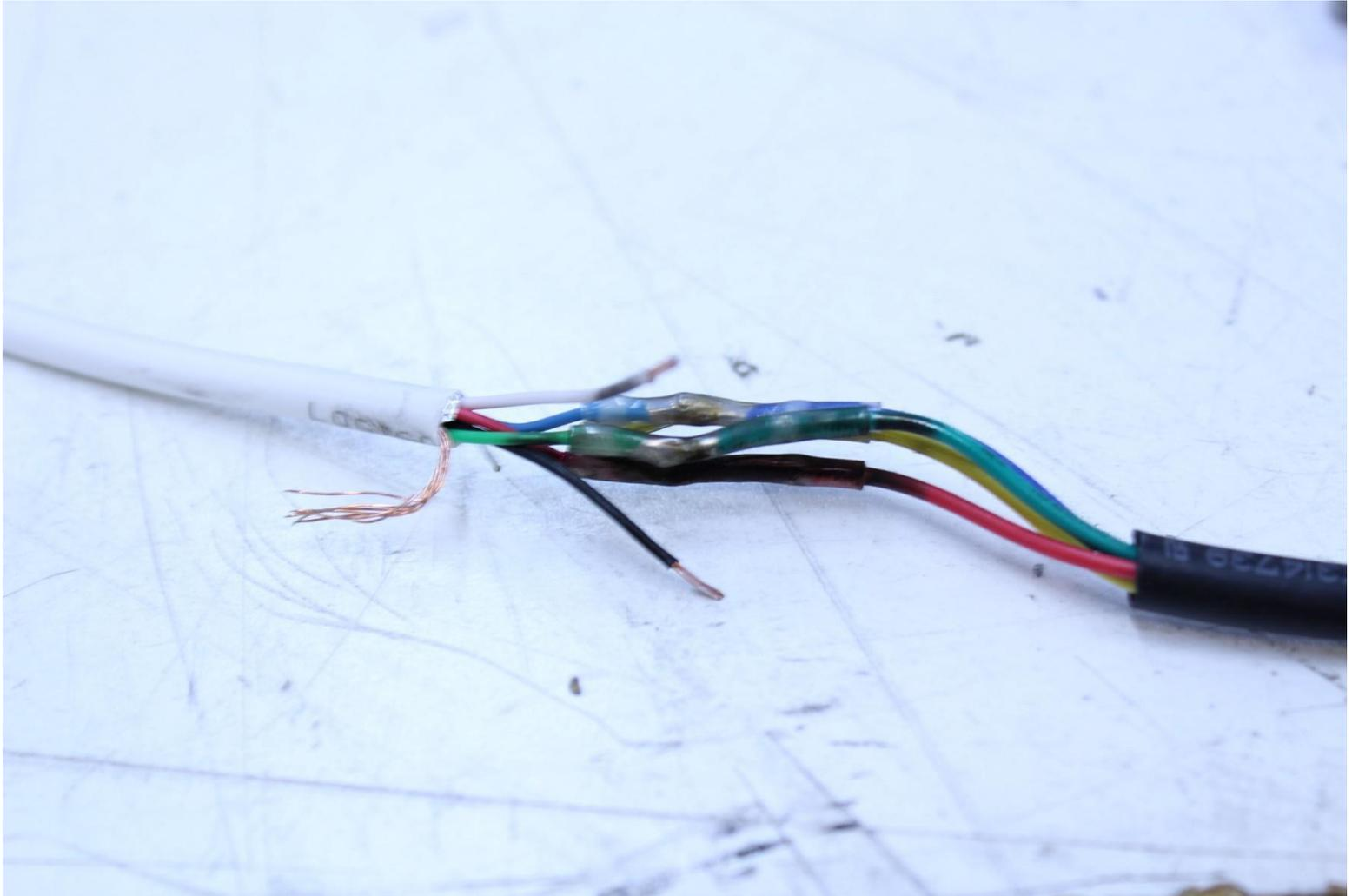
Once all four connections are made, repeat the same for the limit switch attaching them to black and white wires.
