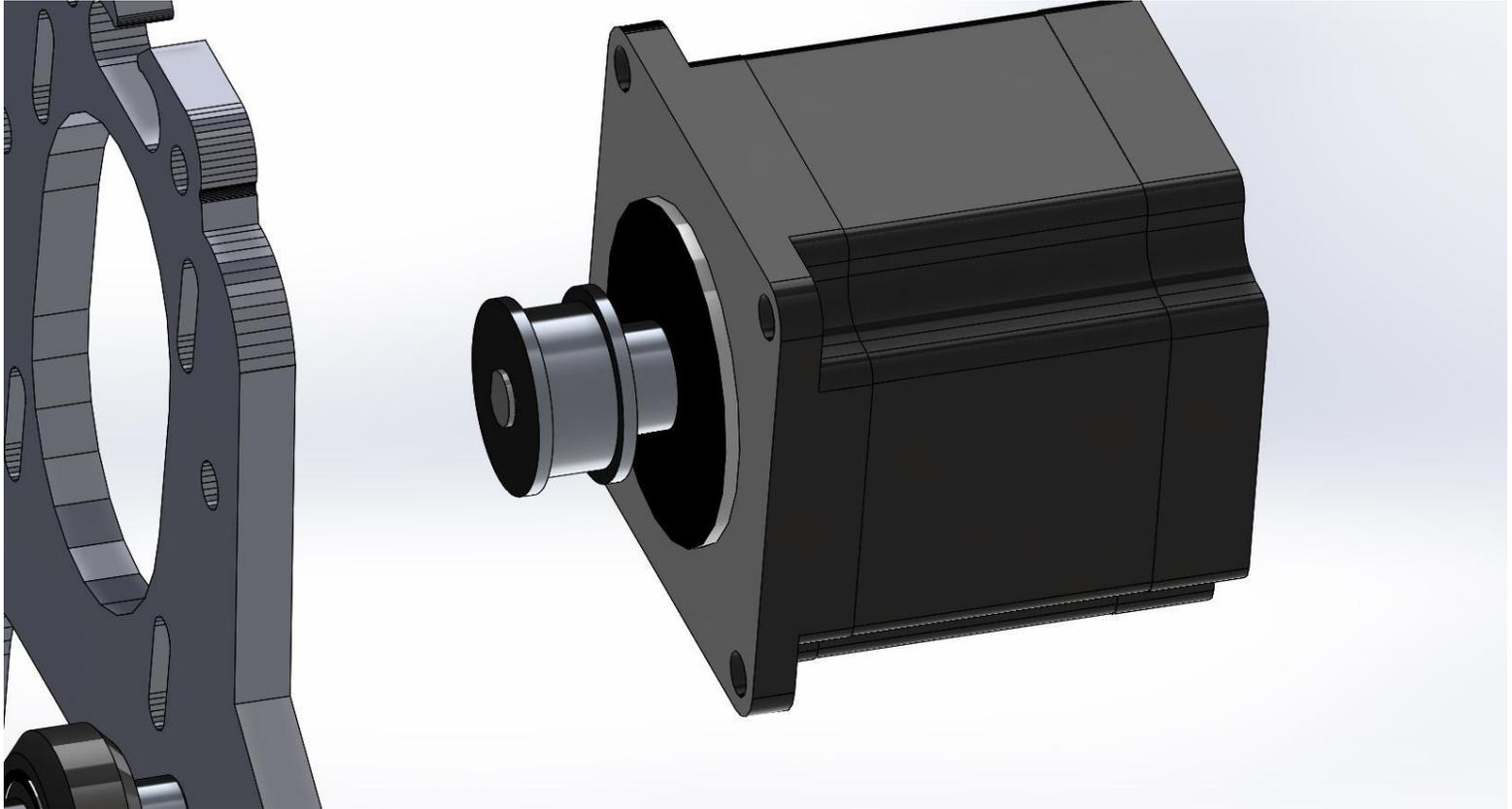
Install the motor onto the rear gantry plate. This is done with four qty M5 x20mm bolts and 4 qty M5 nuts.
