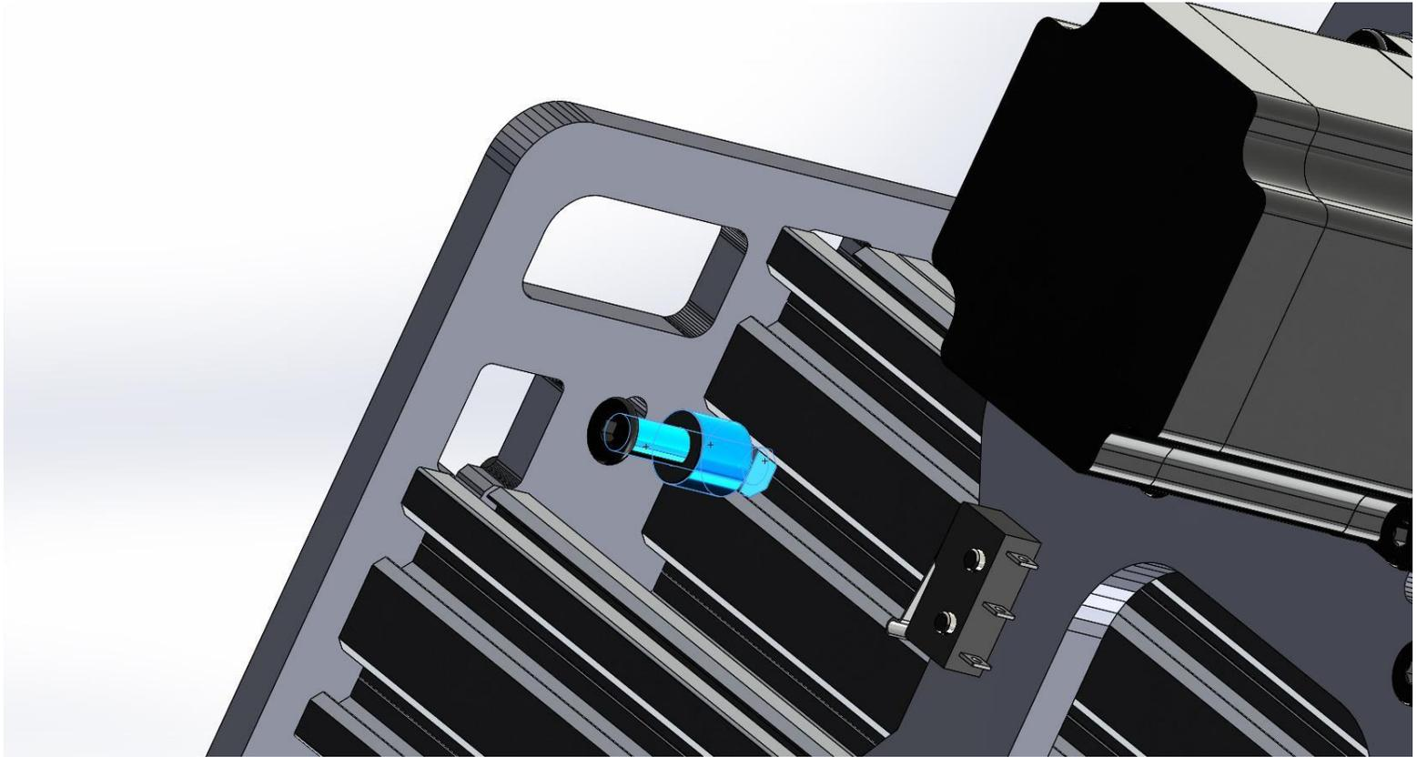
This can always be adjusted later, tighten the bolt down for now in the approximate location shown above. The limit switch arm should contact the 20mm spacer.
