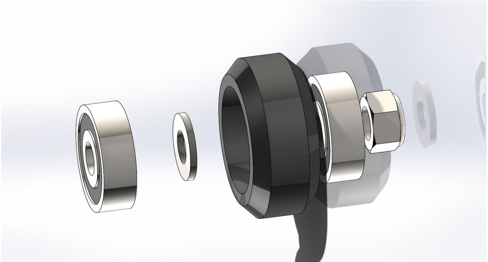
Bearing, shim, wheel, bearing. In some instances, the additional shim is required outside the wheel, the extra shim is not used in this build. Do not use both shims inside the wheel. If the additional shim is required, the build instructions will indicate where to put them.
