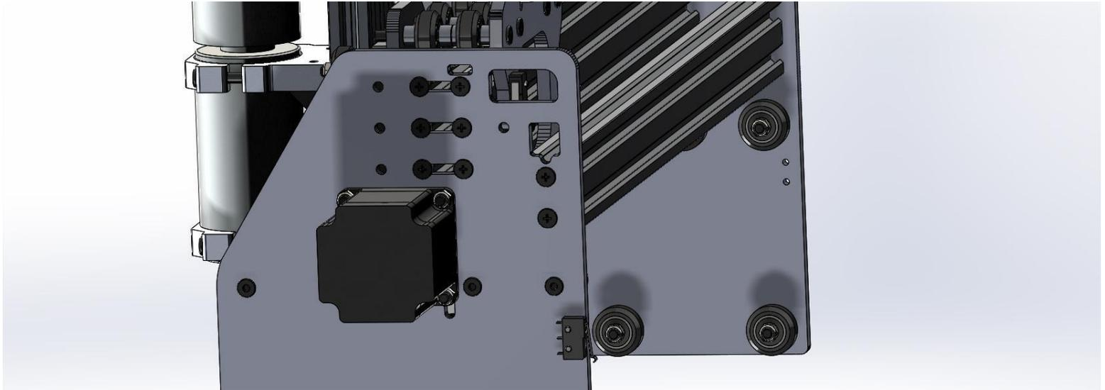
Next, install a NEMA 23 Stepper motors on each Y gantry plate with M5 x 20mm bolts ad secure with M5 nuts.
