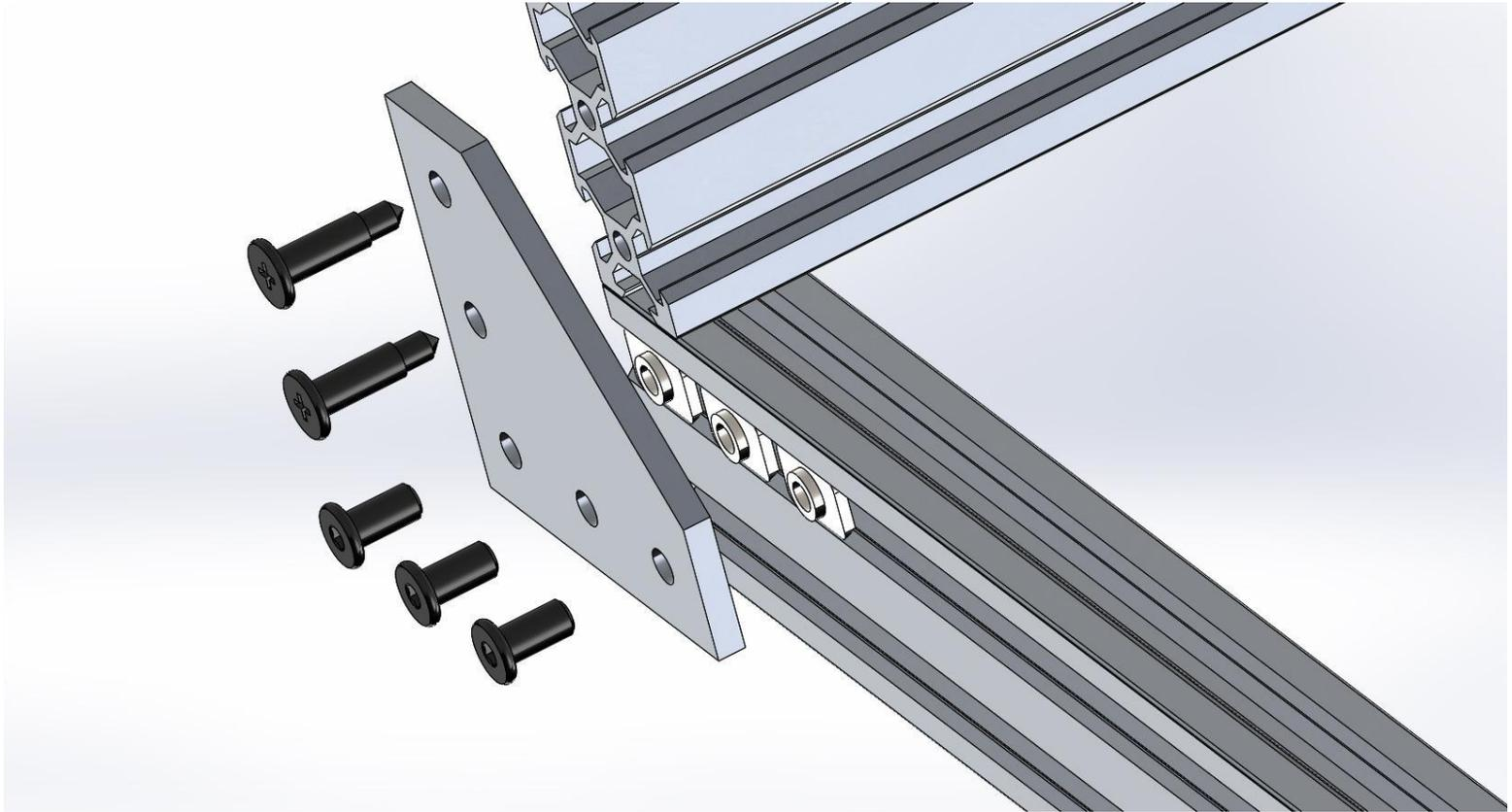
Use a speed square or some device that has a known good 90-degree angle and true the corner of the build, then tighten the screws down on all four corners.
