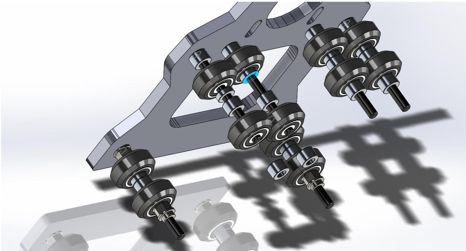
Install the X\_Z assembly onto the front of the bolts and loosely tighten the M5 nuts to hold everything together. Do not snug the nuts down to the front of the X\_Z plate yet as it will make installing the extruded aluminum difficult, we simply want to hold the assembly together.
