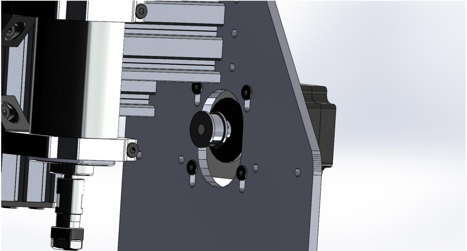
Install the upper wheels on the Y gantry plate with .25" spacers. The lower wheels get installed with .25" eccentric spacers. The bolts are installed with M5 x 30mm bolts and M5 nuts. Again, turn the eccentric spacers to give the most room.
