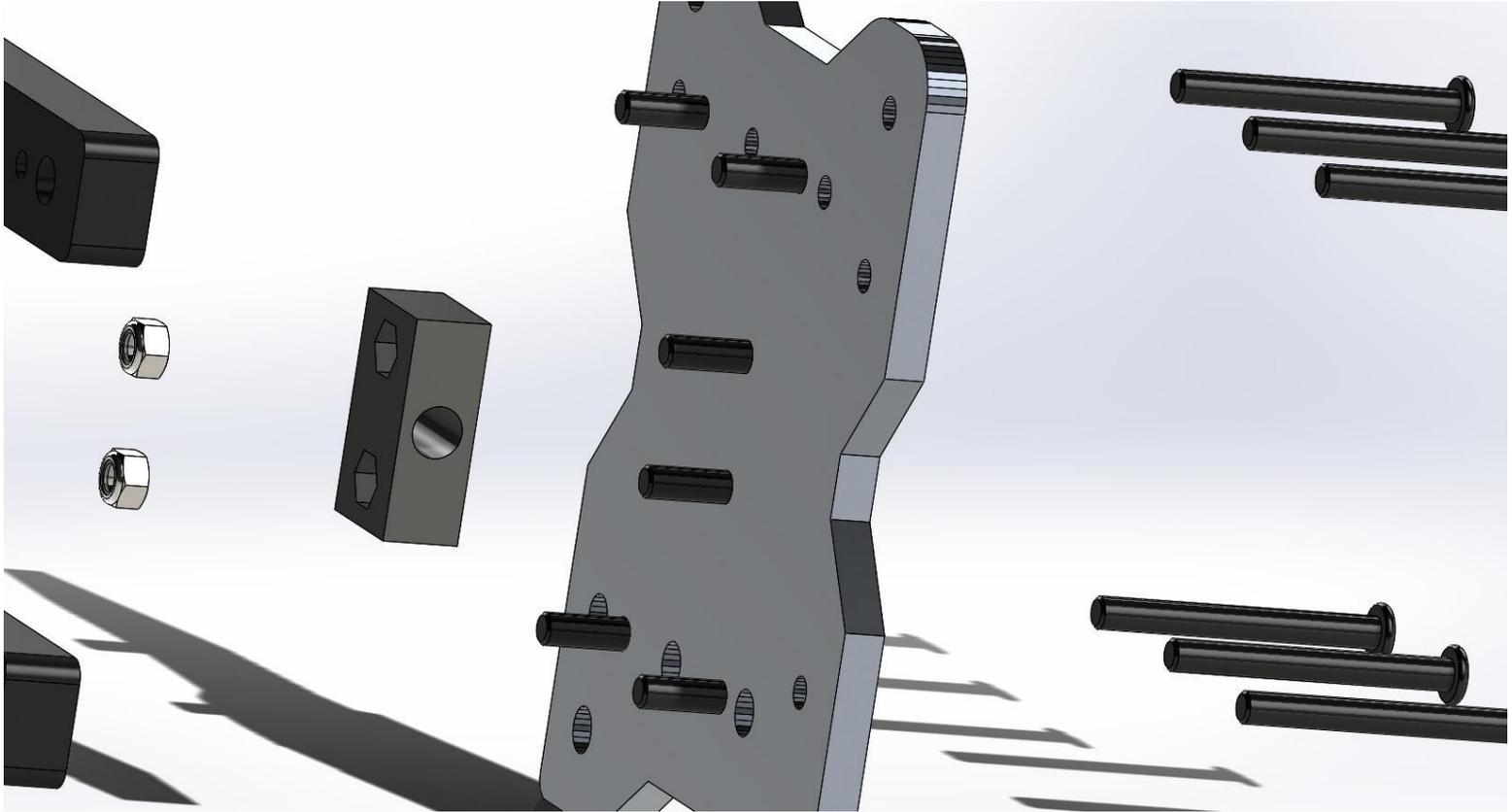
**\*NOTE:** We added a Z limit switch during the writing of these instructions. The gantry plate has since been modified in shape. The sharper corners face towards the bottom of the Z axis. The limit switch should be installed on the side of the plate that the bolt heads (not threads) are on. The images used will show the old profile of the plate in some instances, such as above.
