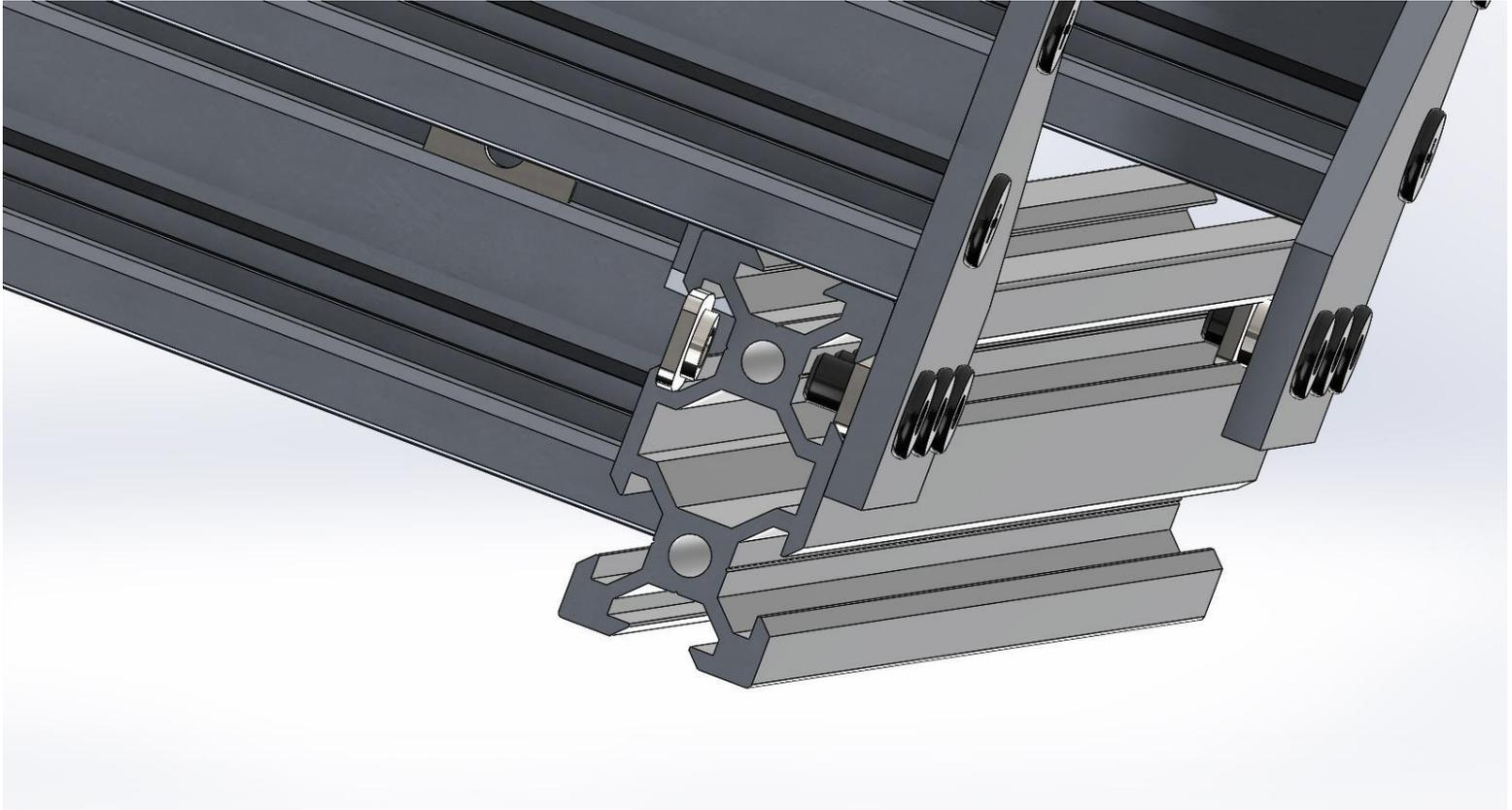
Install all cast 90 degree brackets by M5 x 8mm bolts, square and tighten. 8 qty M5 x 8 used in this example here.
