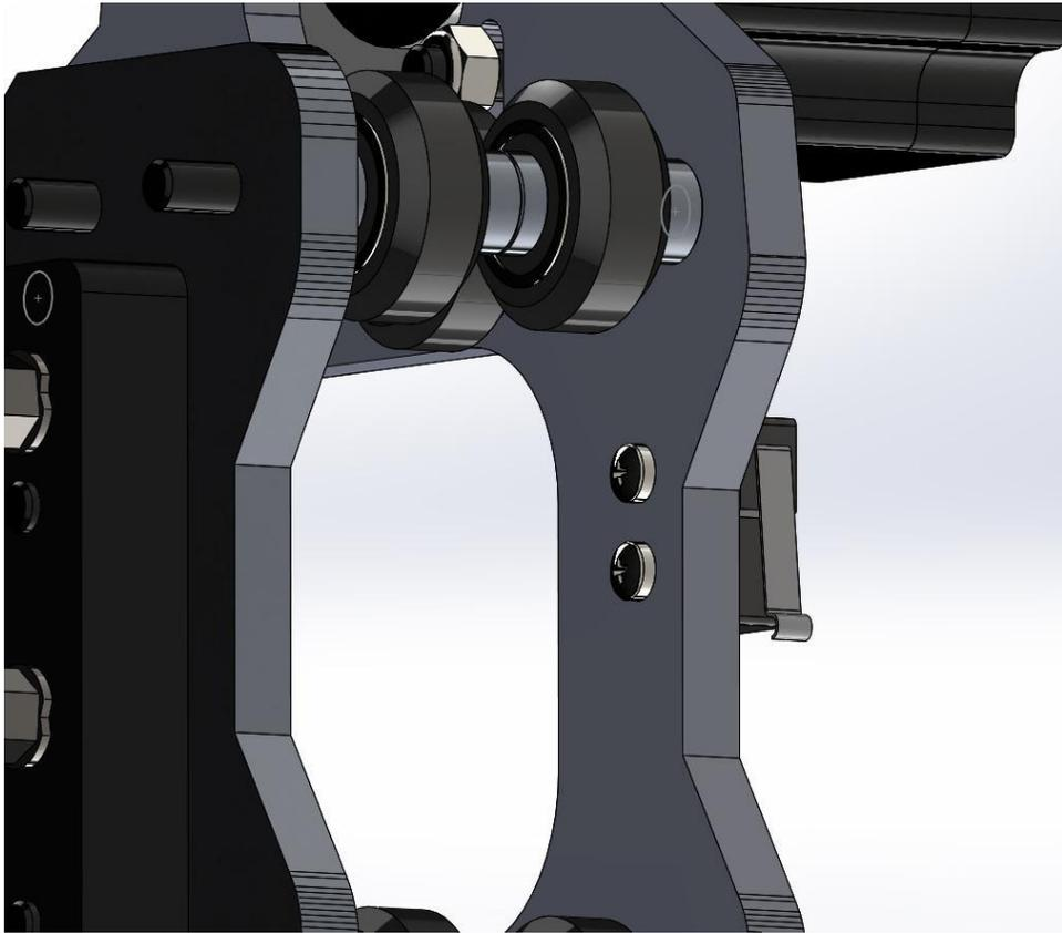
The rear X gantry plate will receive six qty M5 x 65mm bolts. Slide these through the rear plate as shown. Slide a .25" spacer over the top bolts, and .25" eccentric spacers over the bottom bolts.
