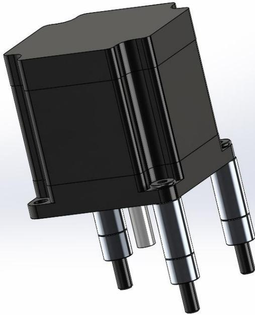
10. Now slide the stepper motor shaft into the coupler and run the three bolts into the matching holes in the threaded rod plate.
