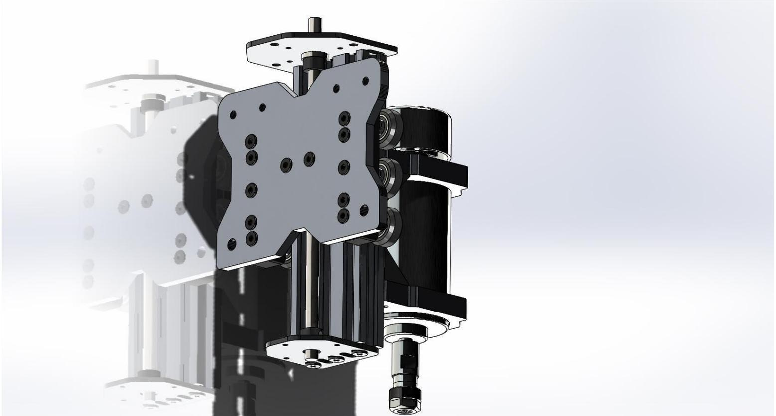
7. Check to make sure there is little to no play when you turn the ACME by hand. Also check to make sure the ACME does not bind when turning by hand. If it does either adjust the lock collars or threaded rod plates to remedy this.
