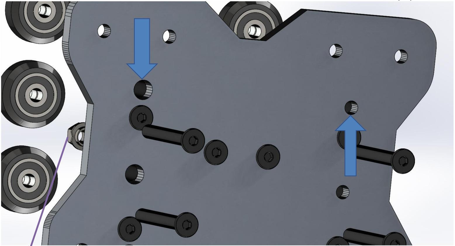
7. Install the eccentrics with the cut-out (on the flange of the eccentric spacer) facing towards the outer edge of the plate.
