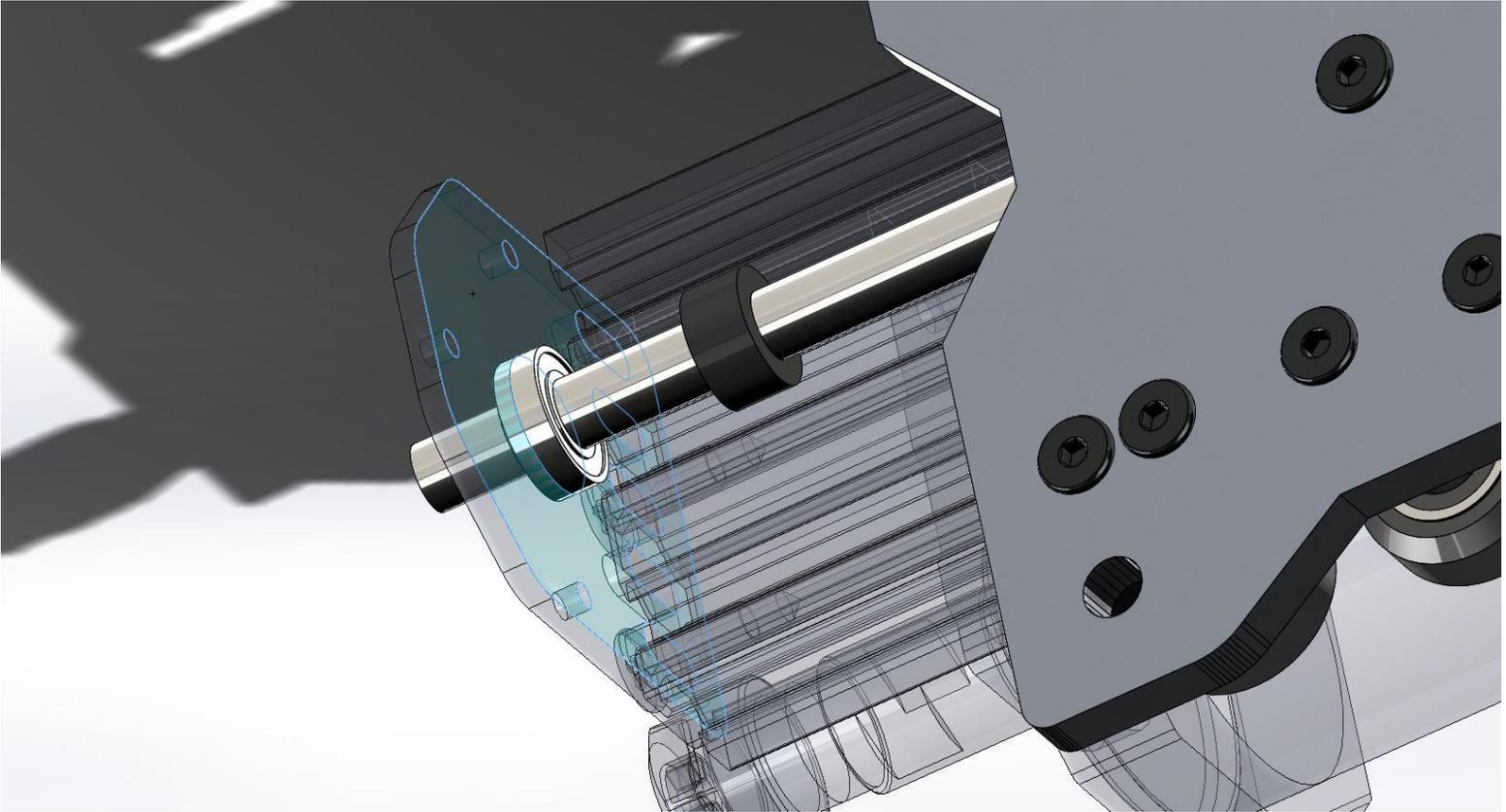
6. Once the threaded rod plates are tightened down, lock the bearings in place with the lock collars. NOTE: you will need to leave about 2mm of ACME hanging out of the bottom of the lower (smaller) threaded rod plate. The above pictures shows an exaggerated amount hanging out for display.
