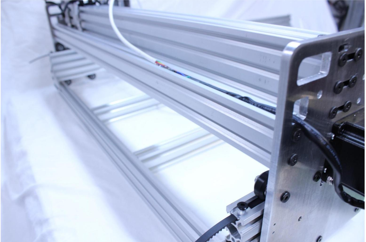
Install the cable chain with a drop-in tee-nut on the 20x40 behind the X gantry and the other end to the rear X/Z gantry plate.
