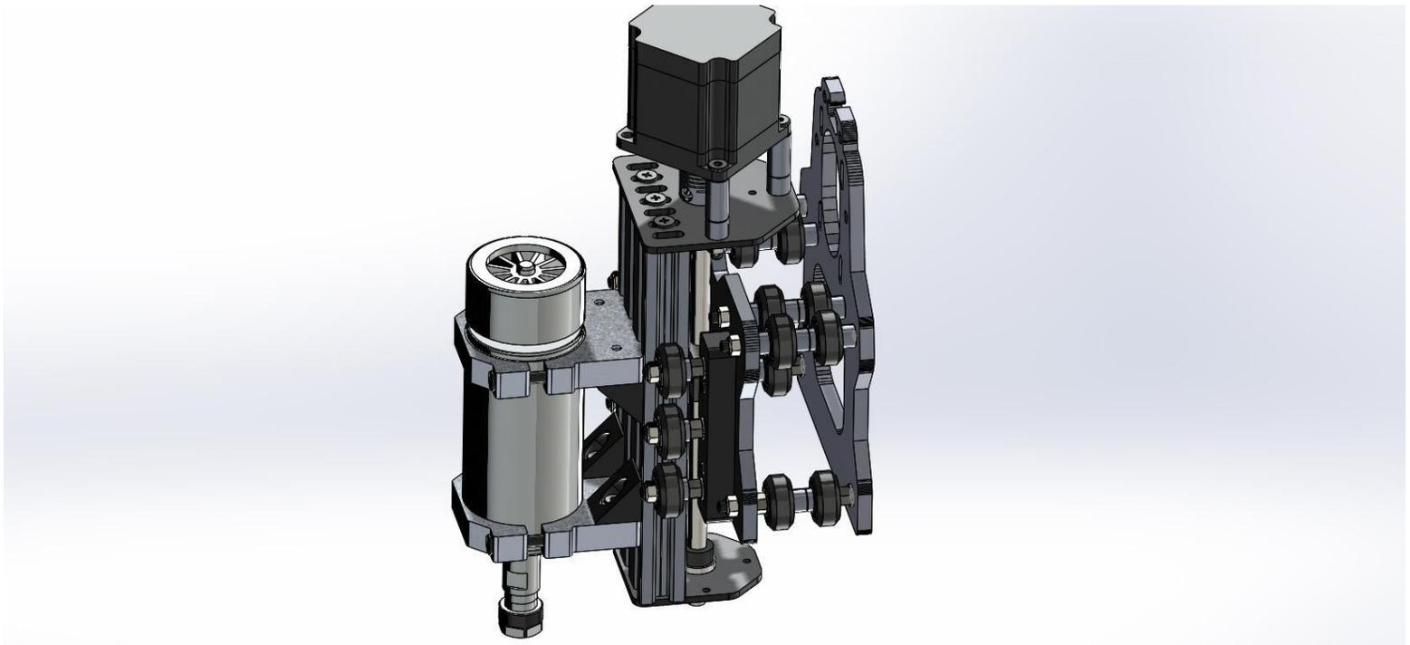
Next install a GT3 pulley loosely onto the NEMA 23 with the shoulder of the pulley closest to the motor.
