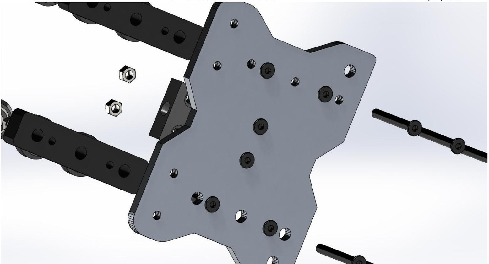
2. Next install 2 qty M5 nuts into the plastic ACME nut block. Note one side has cut outs for the nuts.
