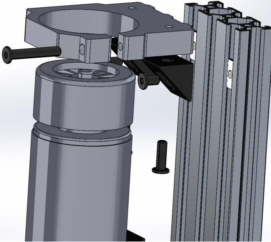
Exploded View. M5 x 8 bolts go into Tee-nuts, M5 x 15 go into V-Slot.
