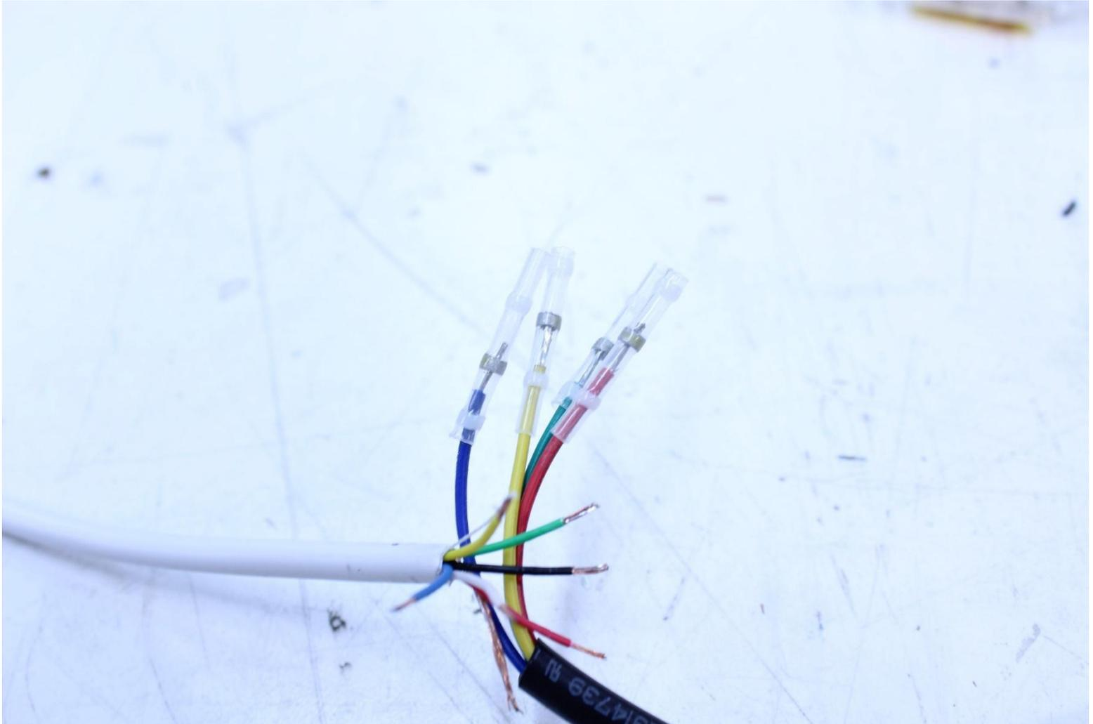
Install so that the tinned wire end meets the inner solder band on the white banded solder connector.
