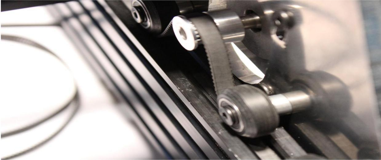
Run it to the end of the gantry and slide a tee-nut over it. Tee nuts are used on the X gantry. Do not over tighten, we do not want to go through the belt with the bolt, just snug against it. Use an M5 x 8mm bolt.
