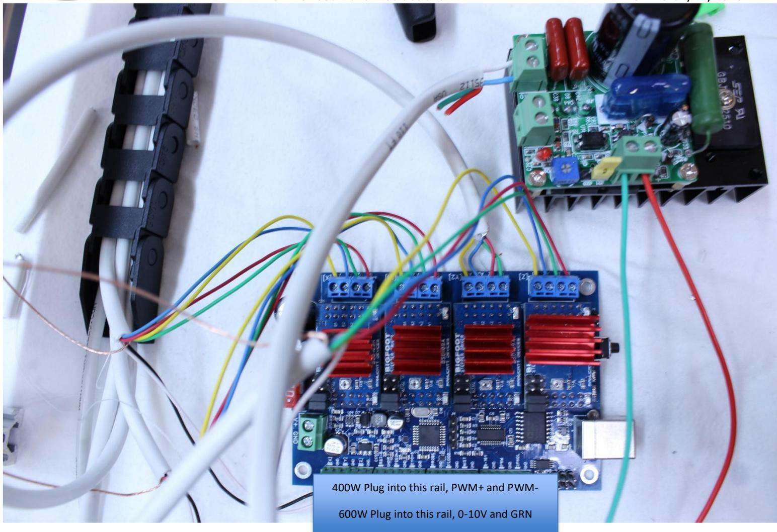
Connect the power supply to the controller and spindle speed control
