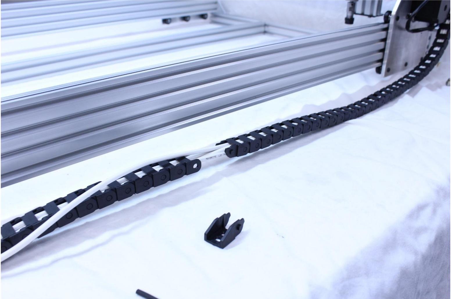
Attach the cable chain to the Y gantry plate threaded hole (9mm spacer, 15mm bolt) as we did earlier on the rear X/Z gantry plate. Attach the free end to the table with a wood screw.
