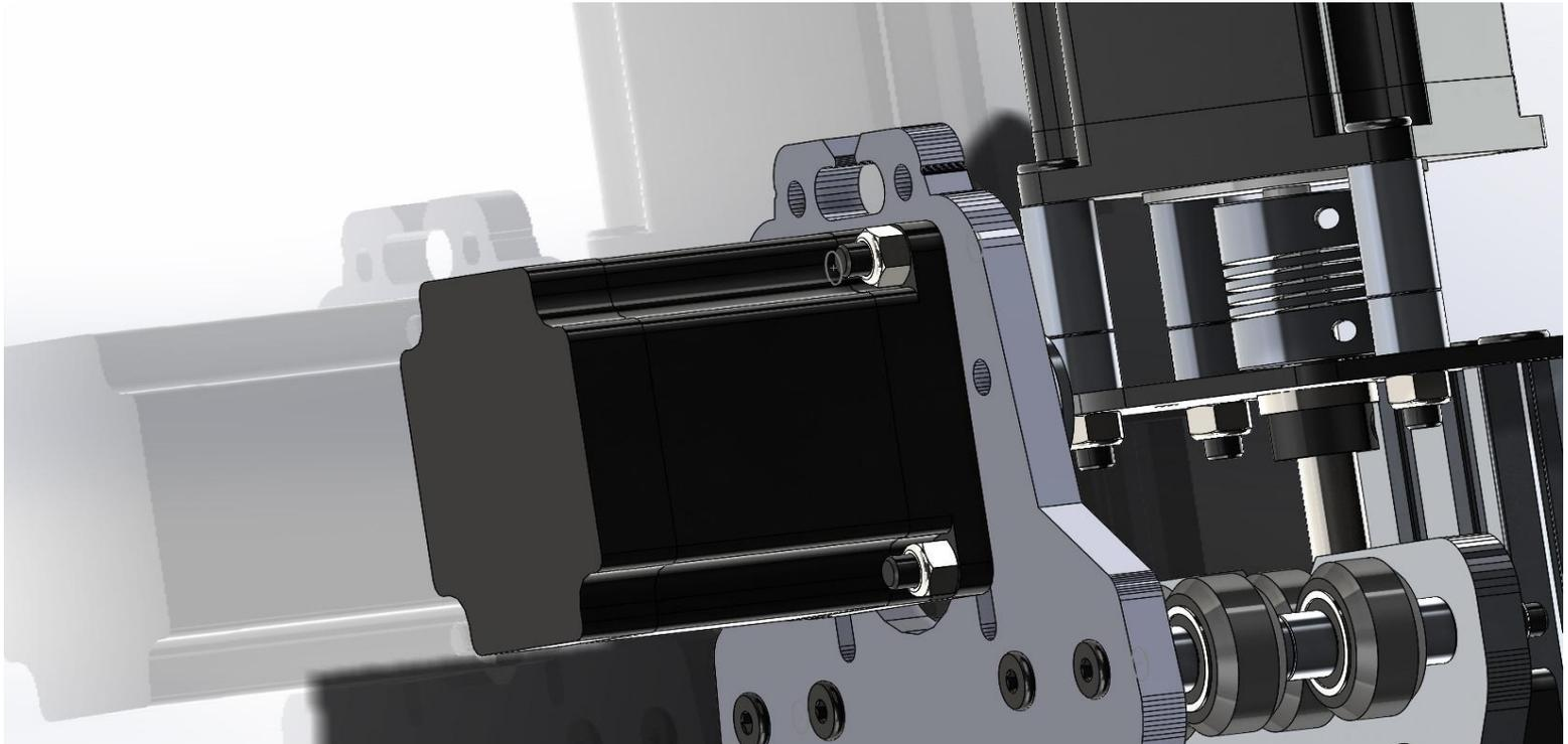
The GT3 pulley should be a distance away from the top threaded rod plate by a distance equal to the thickness of a piece of paper.
