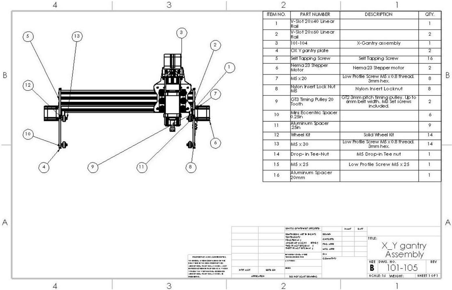
Remove the X gantry extruded aluminum, the length will be based on the kit size you chose. It can be noted which bundle the X is because it contains two qty 20x60 and one 20x40 that are all the same length.
