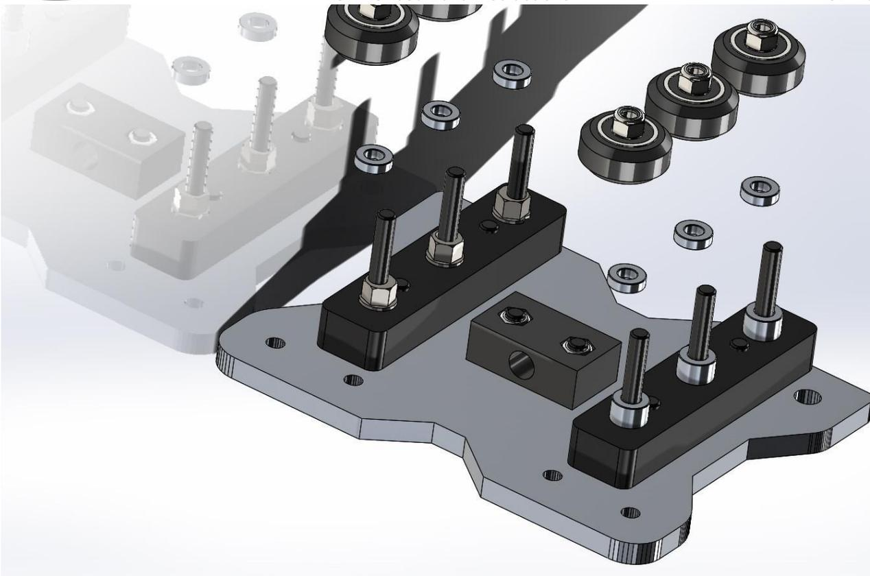
6. Now we will install eccentric spacers on one spacer block and plain spacers on the other. Next install the thinner spacers (3mm) on top of the eccentric and standard spacers. The eccentrics (later) will allow for us to remove slack from the drive. Before installing the eccentric spacers, note that one set of holes on the rear of the X gantry plate is larger than the other. Install the eccentrics on the larger hole set:
