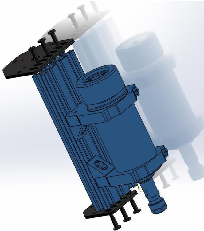
8. The smaller plate goes on the bottom, the bearing recesses (on the threaded rod plates) face each other. Install with 3 qty (per side) self-tapping screws and leave loose. Note, we provide a screw driver, but the self-tapping screws are much easier to set with a drill motor.
