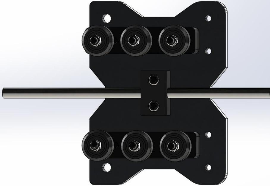
2. Install a 688zz bearing and lock collar on each end. **Reverse order shown below, lock collar goes on first.**
