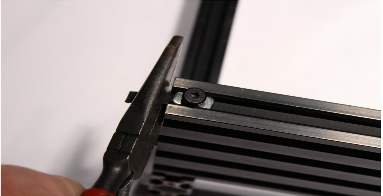
End of the Y gantry shown above, give it a good pull and tighten the M5 bolt in the tee-nut. Don't get too tight! You can go all the way through the belt if not careful, we do not want to go through the belt, just snugly against it.
