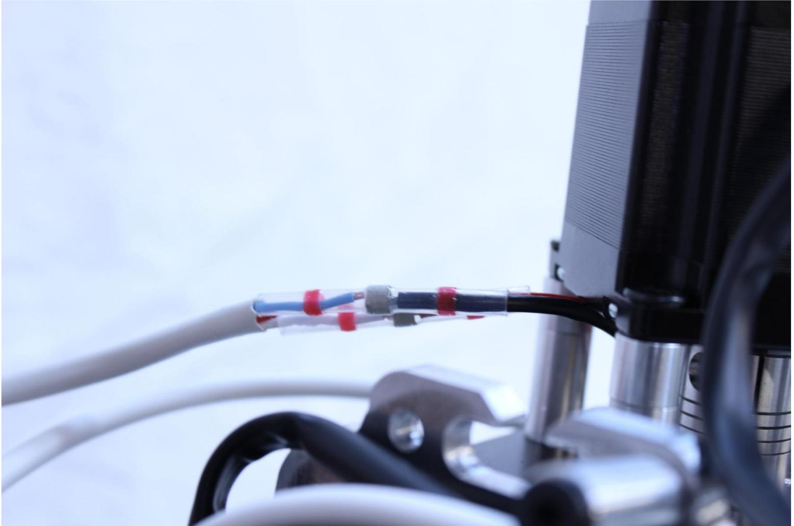
The opposite side Y should run under the cable chain and jump through the bottom of the cable chain prior to exit.
