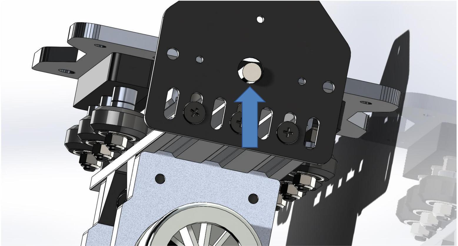
4. Next, with the screws loose on the threaded rod plate, we will align the bearings with the recesses in the threaded rod plate.
