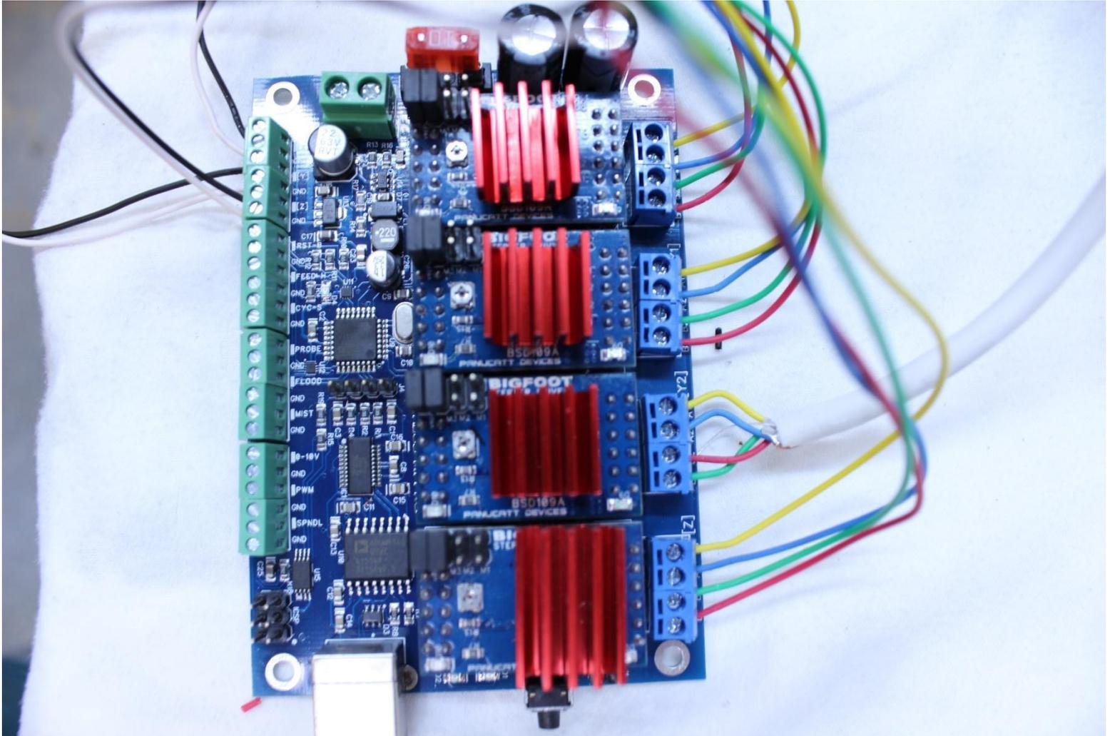
X goes to the top connector, Y then Y, then Z is the bottom. The colors of the wires are important! Connect them just as shown here. The limits will wrap around the other side and are (from top to bottom) X,Y,Z. Notice how the second Y motor has a reversed connection.
