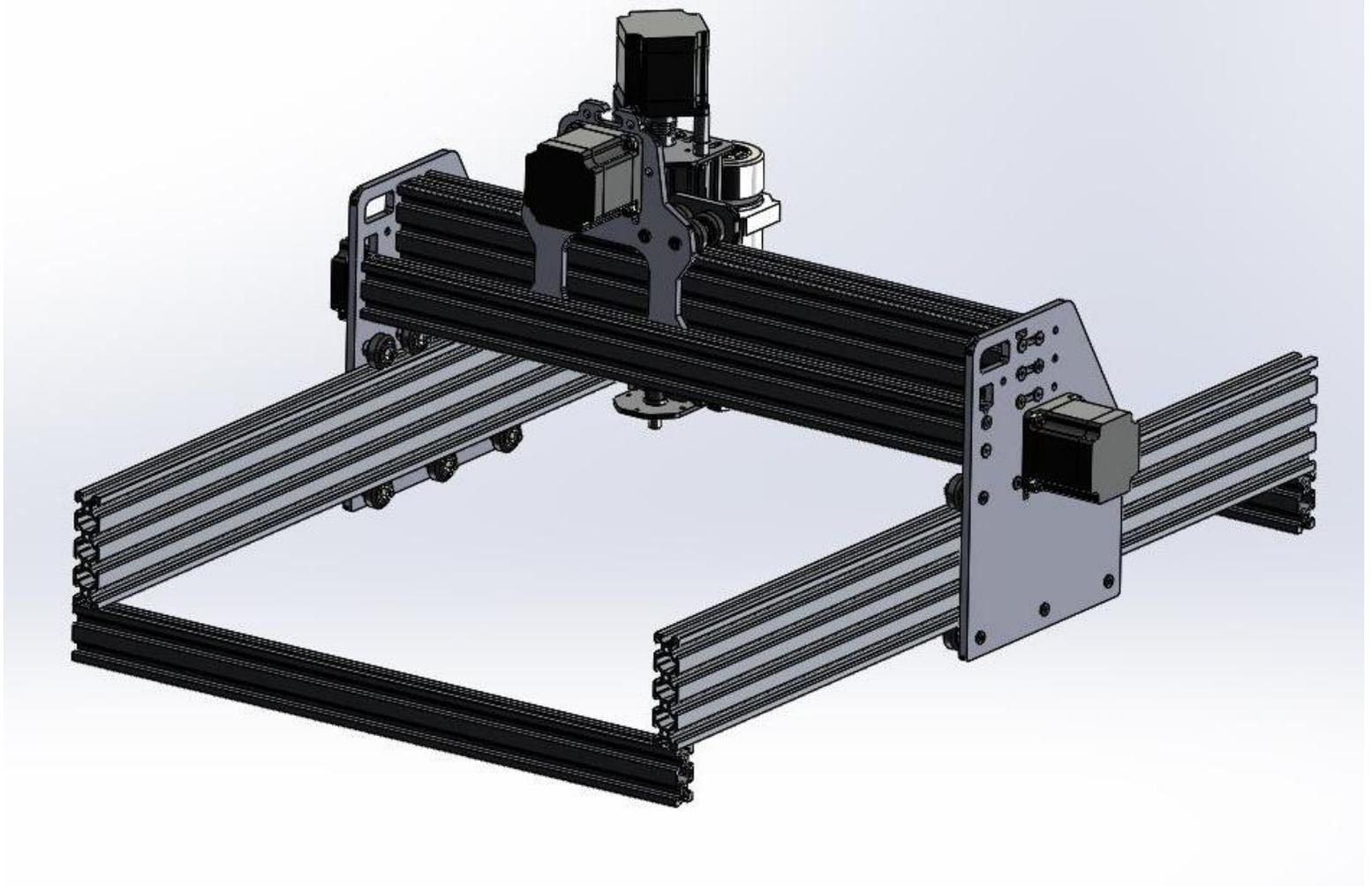
Using the 5-hole 90s from this step install them between the 20x80 and the 20x40. Use Tee-nuts with M5 x 10 bolts in the 20x40 and self-tapping screws in the 20x80.
