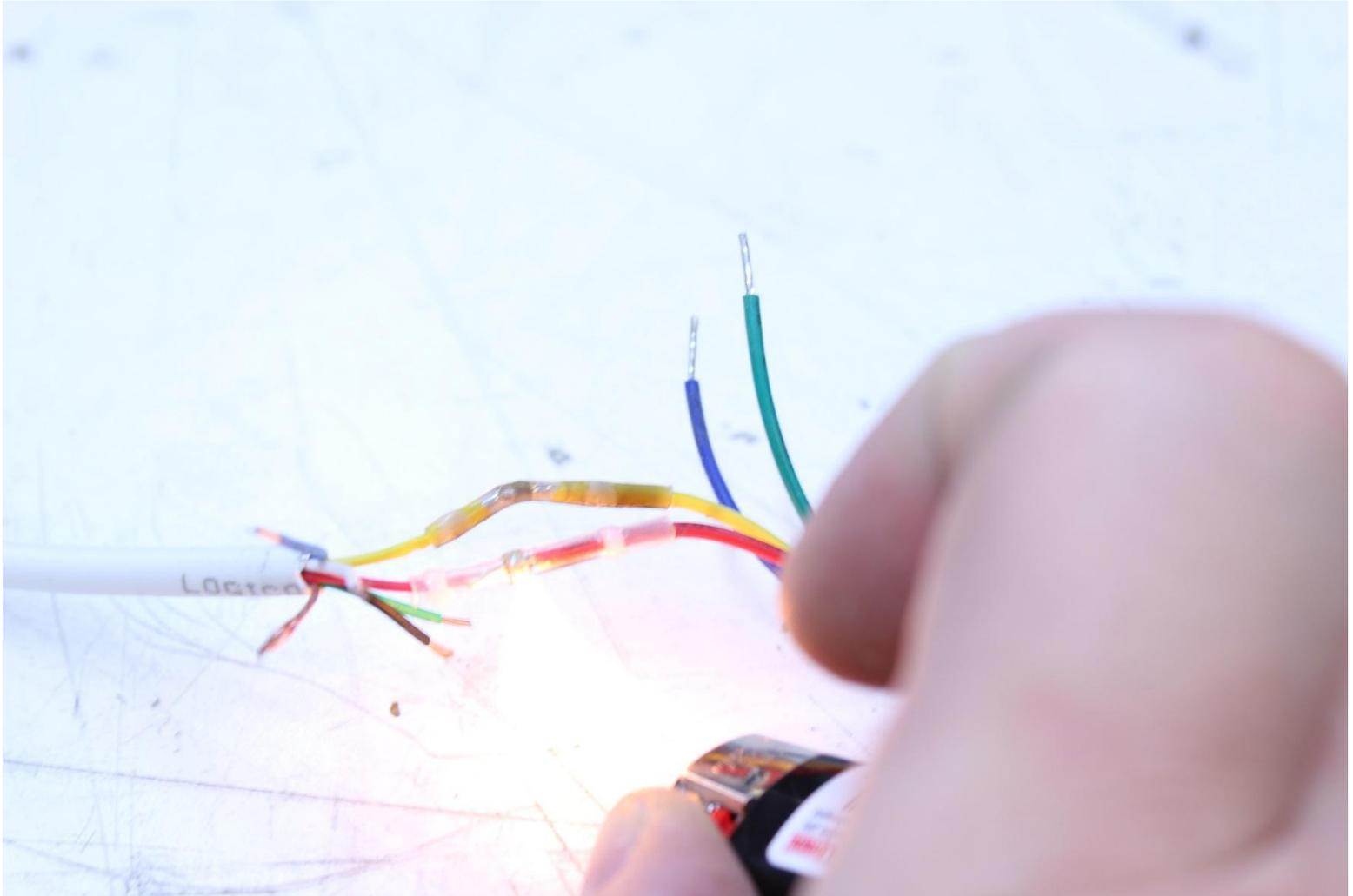
The yellow connection in the image above is complete, the red is in process of melting.
