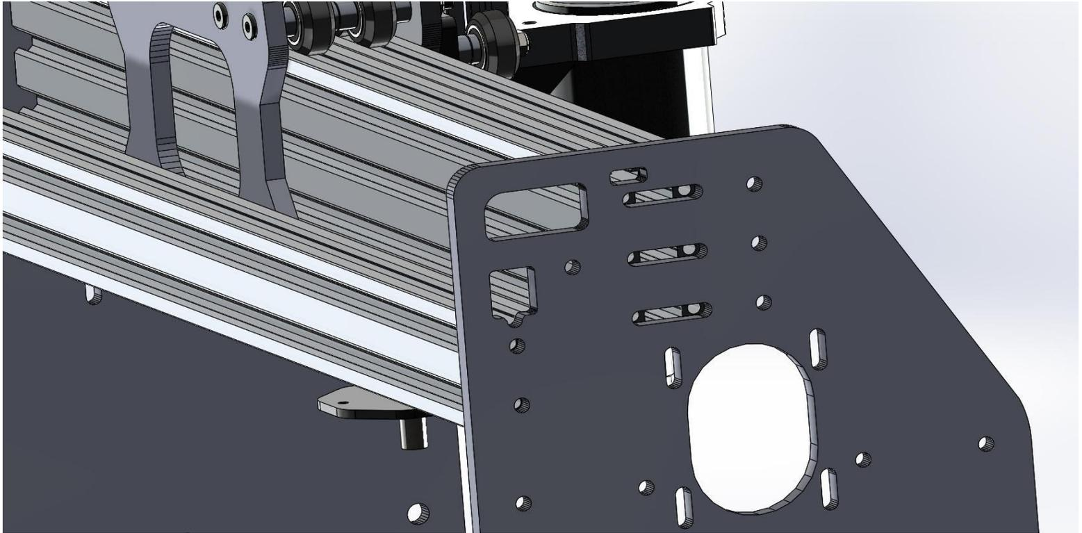
Note: Limit switch stop can be added here. A drop-in tee nut, M5 x 30mm bolt, and 20mm spacer will be assembled and inserted here. On the back of the 20x60 on the LH rear side, about 20mm (~1") away from the gantry plate install in the middle slot:
