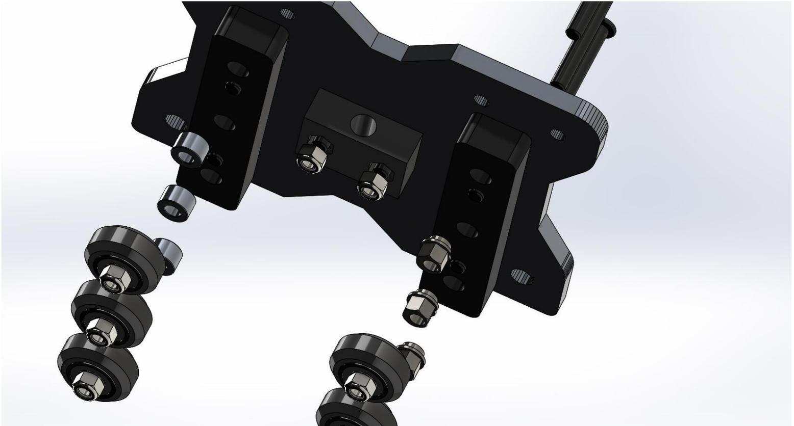
3. Tighten the M5 x 20 bolts holding the black plastic ACME nut block on, snug, do not crush the plastic nut... it is possible! The bolts need to be tight, not torqued.
