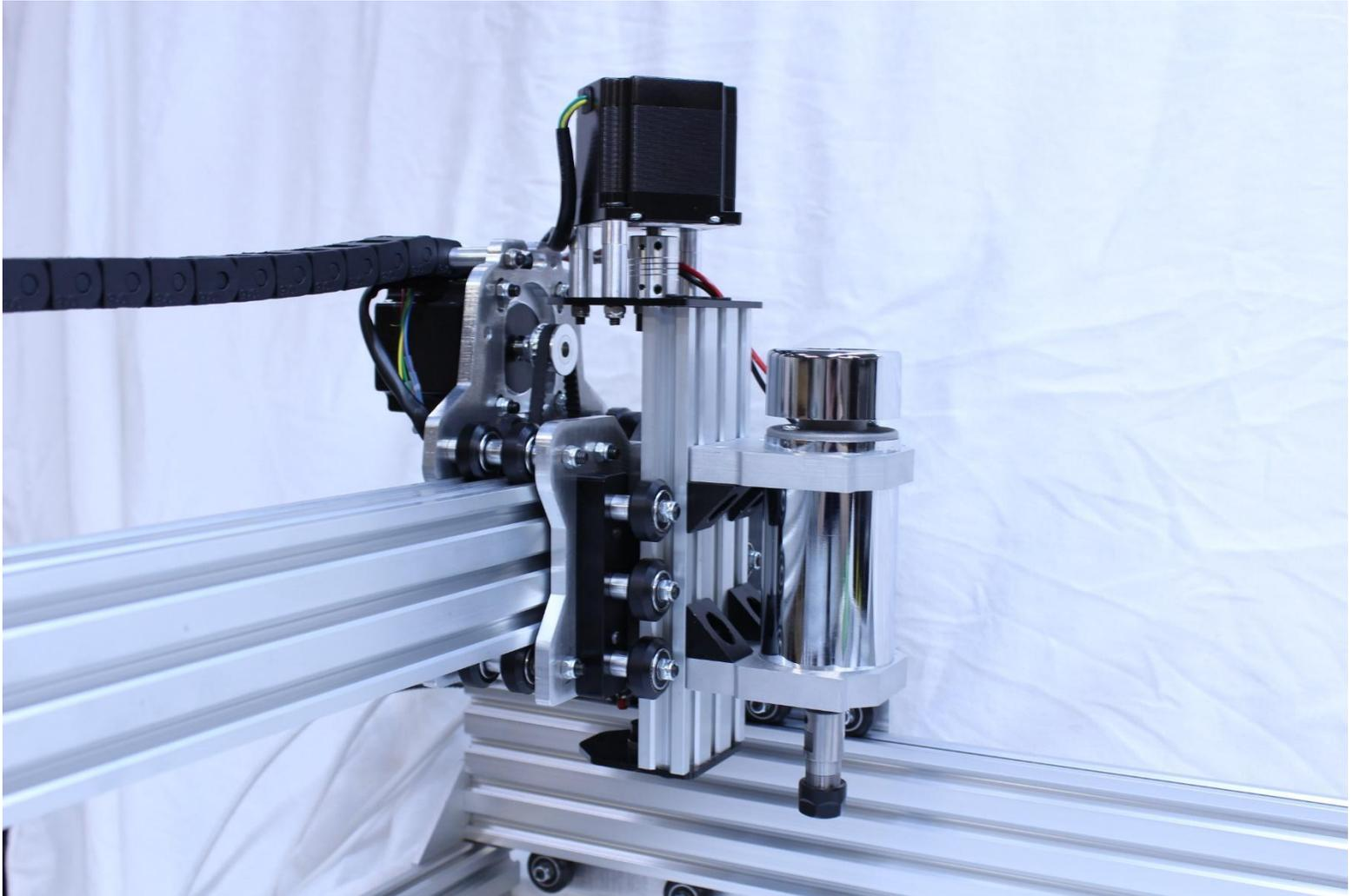
Now, coming out of one side or the other Y gantry plate you should have wires that are connected to the X, Z, and opposite side Y motors and limit switches.
