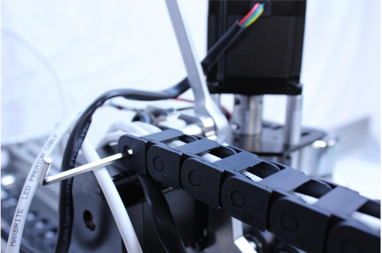
The other end will lay on the 20x40 and is installed with a drop-in tee-nut:
