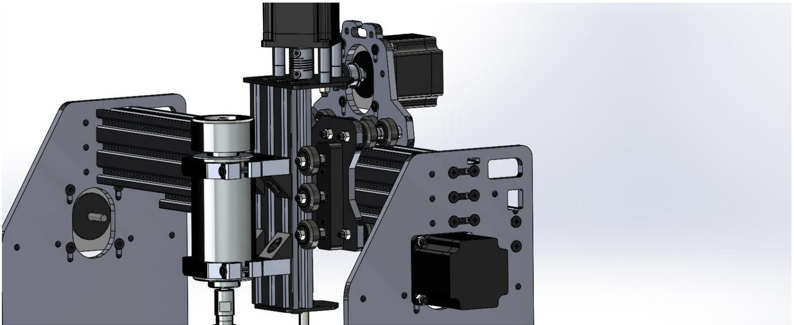
Install the GT3 pulleys on the NEMA 23 stepper motors. Leave the set screw loose for now. After installing the belts in the final Y assembly, align the pulley with the belt and tighten the set screw.
