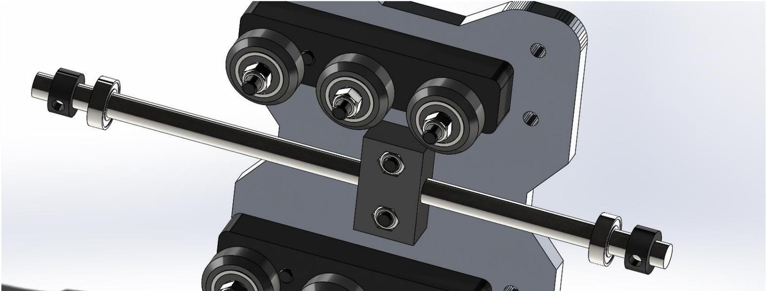
3. Position the Z axis from step one (with one removed threaded rod plate) over the wheels and slide into place. Be cautious of the tension between the wheels and the 20x80, if it is too tight make sure the eccentrics are properly placed.
