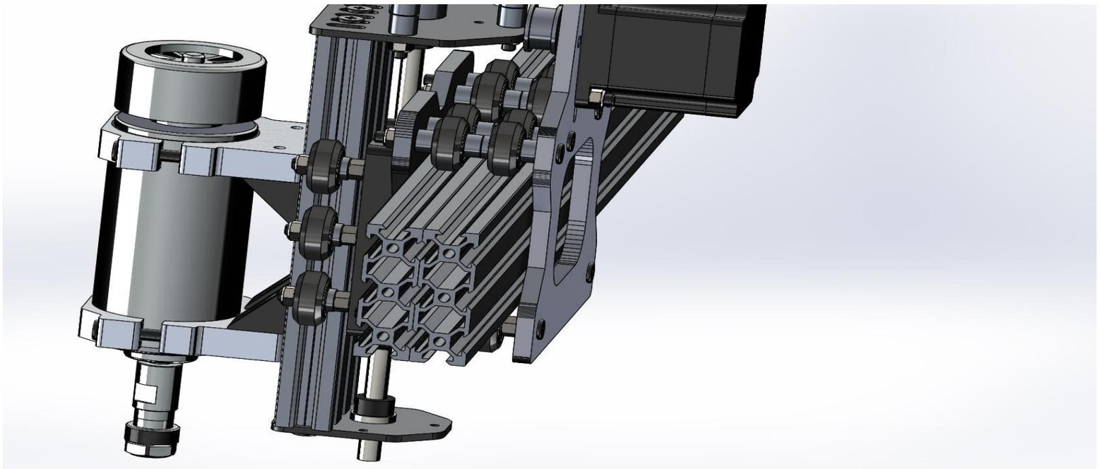
Install a Y gantry plate on the end of the 20x60s using self-tapping screws. Follow with the rear 20x40 before completely tightening the self-tapping screws. IF the rear 20x40 is short you have mixed the bundles of aluminum. Look for the 20 x 40 that exactly matches the 20 x60 length.
