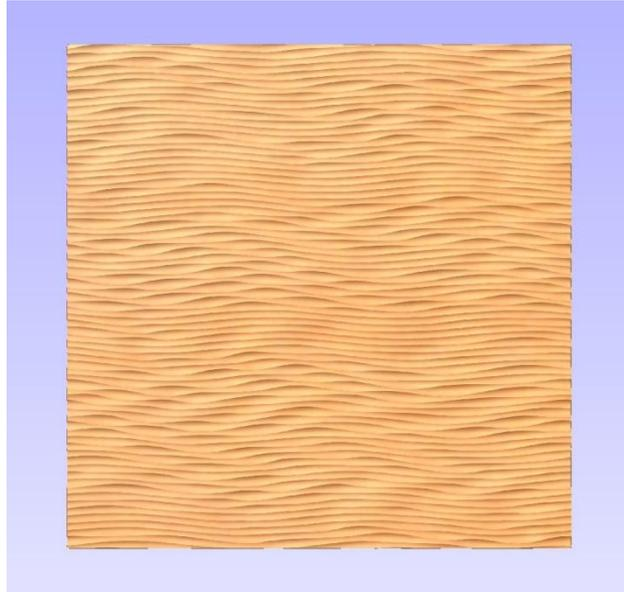
The images below show Maximum Groove Height = 0.800", 2 Wobbles per Line, Amplitude=30%, Progressive Wobble Shift checked (left) and un-checked (right).
