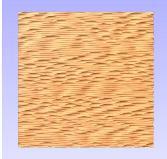
The following image shows the effect of increasing the Wobble Amplitude to 50%. In this case, the Layer 3 sausages went below  $Y=0$ , so I increased the Y borders by 1.0" (top and bottom) in **StandingWave**, and increased the material height in VCP by 2.0".
