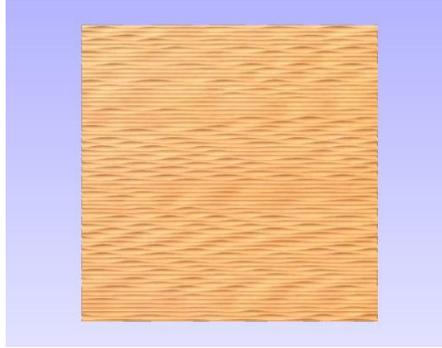
Increasing the Maximum Groove Height to 0.800" increases the contrast, and makes it less likely to find long bands extending across the entire panel.
