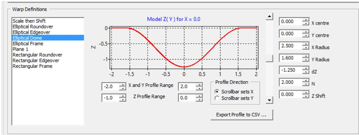
e) Run the **WarpDriver** to create the CSV file, and save this. I put in 4 roughing passes to reach the 1.25" bowl depth. Save the CSV data, and load it into VCP with the CSV gadget. (Too many Three-Letter Acronyms !). Here is the preview. The smoothness of the surface is much better than what I can do with flutes, and it makes the image difficult to see.
