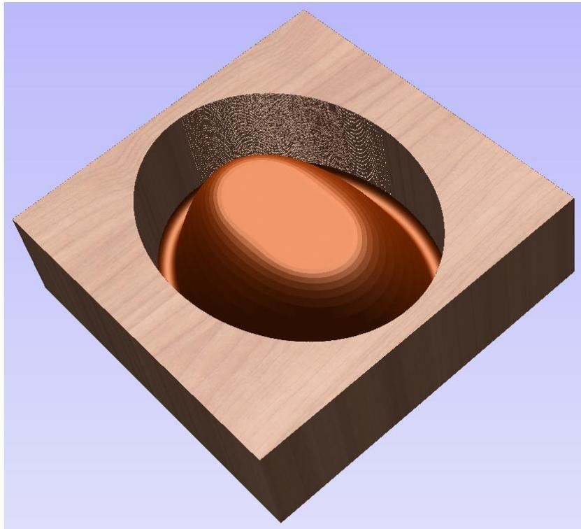
**Second Route : You design the concave and convex shapes in WarpDriver, using the zero-depth pockets described in the WarpDriver manual.**
