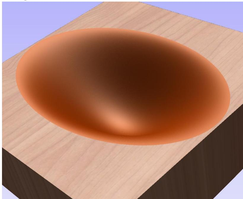
f) repeat the process to create the outer surface, using an convex dome with  $dZ=1.25$ . You can imagine several different designs, but I am going to use the same shape but shifted so that at the rim there is 0.25" of material left. Keeping all parameter the same, except for the  $dZ = 1.25$ . Make the CSV data, and load it into VCP.
