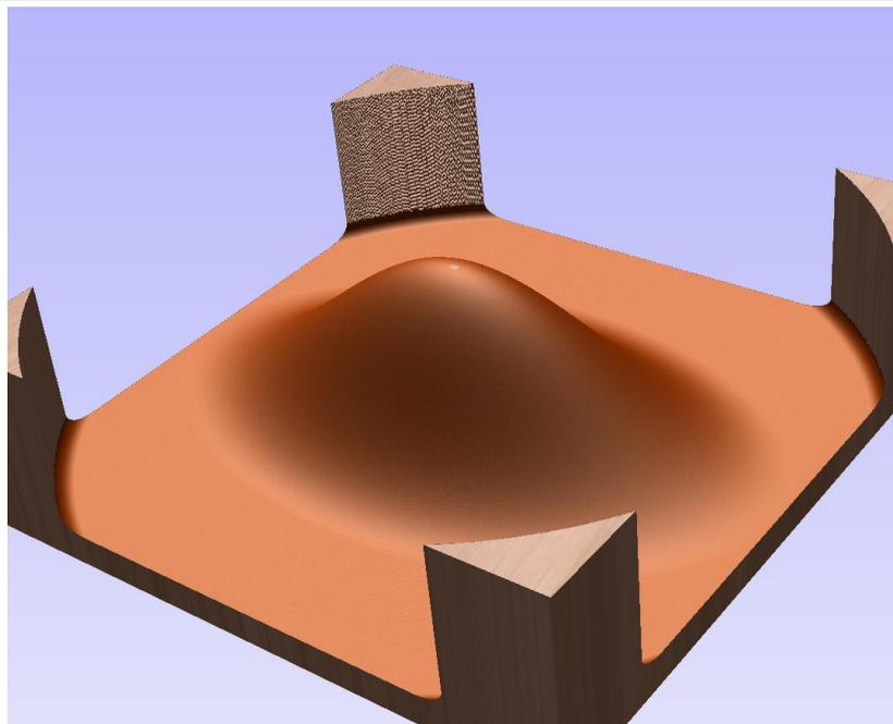
g) The final step would be to do a profile pass to cut out the shape from the bulk material, probably following the 5"x3.2" elliptical shape, using an onionskin to hold it in place.
