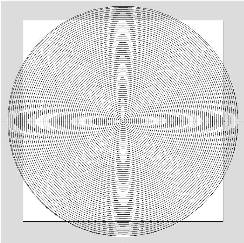
c) Save the gcode to generate this zero-depth pocket, and load it into **WarpDriver**.
